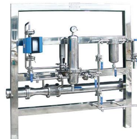
Beerwort oxygen filling setting (Automation was hes belt)
